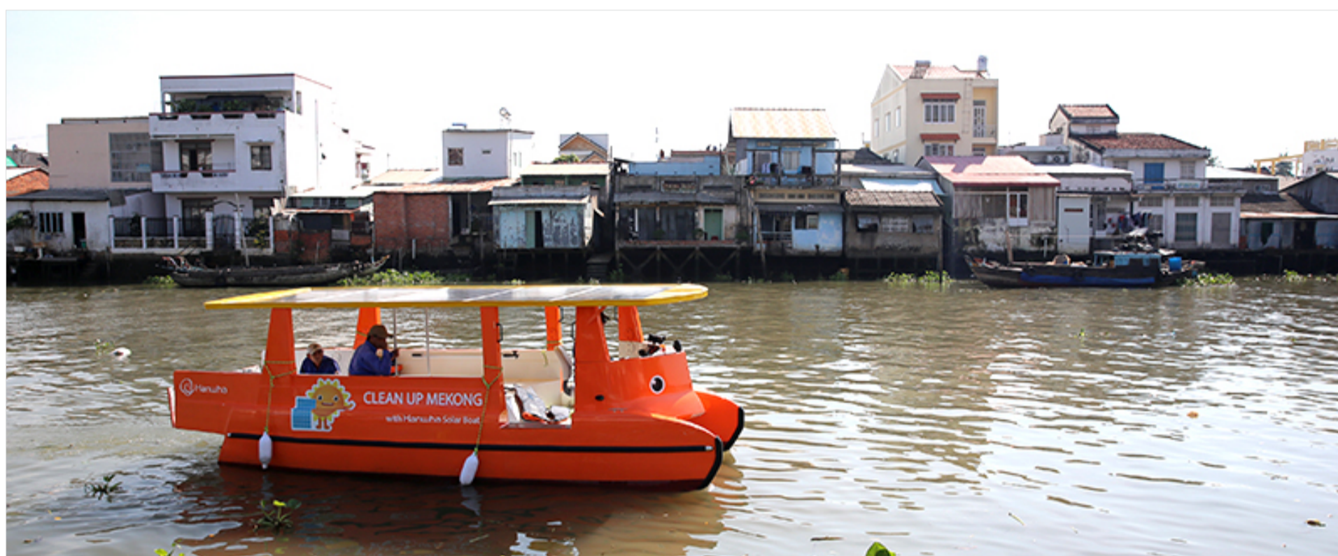
The solar-powered boats donated by Hanwha to the Clean Up Mekong campaign will use conveyor belts to quickly and efficiently scoop floating trash on the Mekong River's surface
