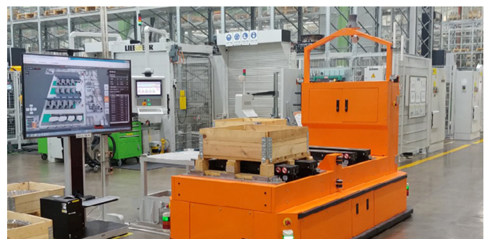
An automated guided vehicle delivers an engine component to a workstation at Hanwha Aerospace’s flagship plant in Changwon, Korea
